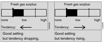
The qualitative assessment of the econometer reflects the prevailing conditions in the breathing system most accurately when anaesthetic ventilation for adults is carried out with a rate of 6 to 25 strokes per minute. The econometer is optimised for frequencies between 6 and 25 strokes per minute - but it can be used up to 40 strokes per minute if a slight instability can be accepted.
