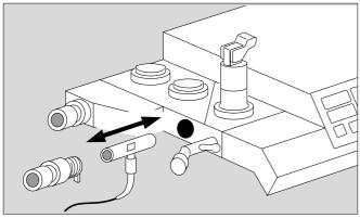
Shake the sensor briefly in the ambient air to purge it of any residual breathing system gases. Tightly seal the sensor openings (on at least one side).
