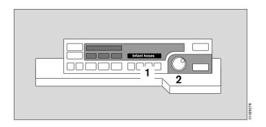
Then switch to »Standby« and call up the leakage test (see page 46) so that the new compliance can be calculated:
