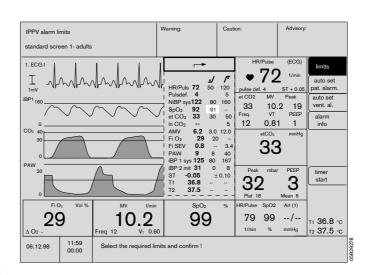
If several alarms occur simultaneously (in this example: pulse rate), the alarm limits which have been exceeded are shown against a dithered yellow background. When the first alarm has been confirmed (by pressing the rotary control on the system screen), the alarm limit of the alarm with the next lower priority is activated and displayed.
