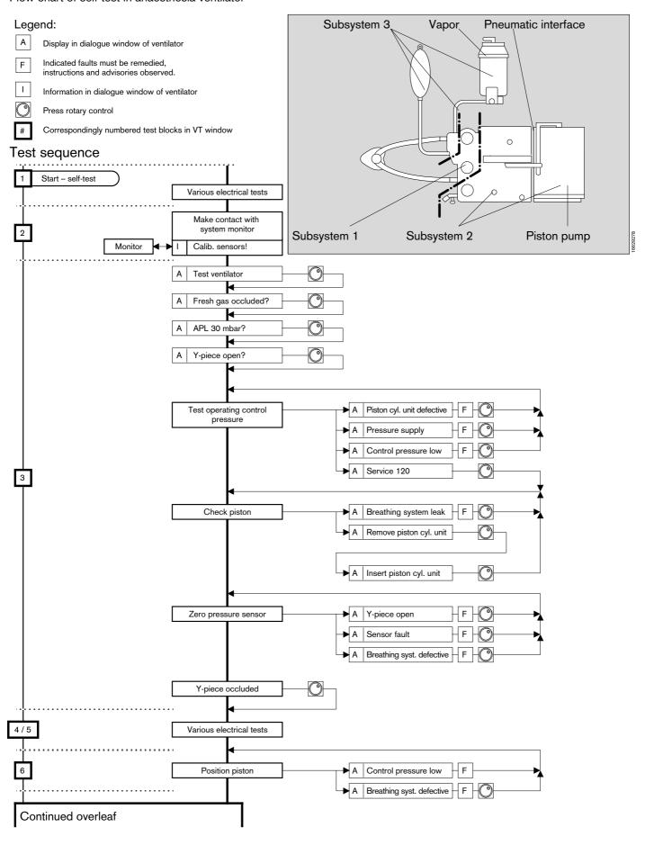
Flow chart of self-test in anaesthesia ventilator (cont.)
