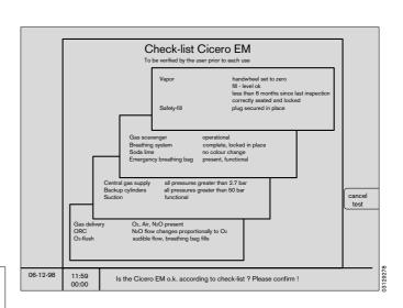
As a basic rule, the general task to be performed is specified in the centre field, and detailed operating instructions to the user are given at the bottom of the screen. The test begins with the question:
