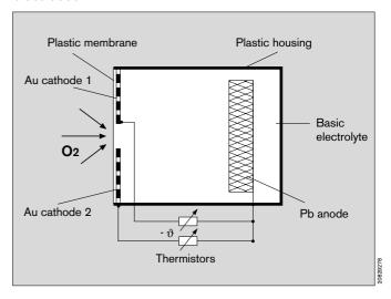
A base electrode is oxidized at the same time. It is depleted by the oxidation process and essentially determines the service life of the sensor. The current flowing through the cell is proportional to the partial oxygen pressure in the gas mixture to be measured.
