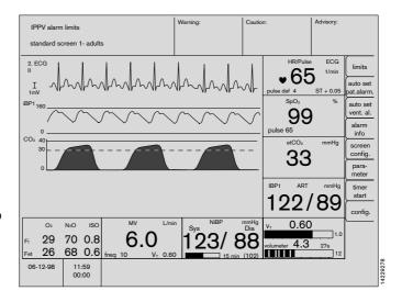
The MAN/SPONT alarm limits are automatically activated in »MAN/SPONT« mode and the SIMV alarm limits for »SIMV« mode with a ventilation frequency of less than 6 breaths per minute. The currently active alarm limits are indicated in the status field and flash for the first five seconds.
