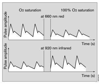
The diagram above shows an example of the light absorbed by the blood at 660 nm (red) and 920 nm (infrared).
