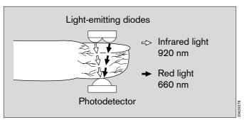
These two wavelengths – 920 nm and 660 nm – are used because meaningful absorption values are still obtained for oxygenated and reduced blood, even in the presence of slight perfusion, and because they differ significantly.
